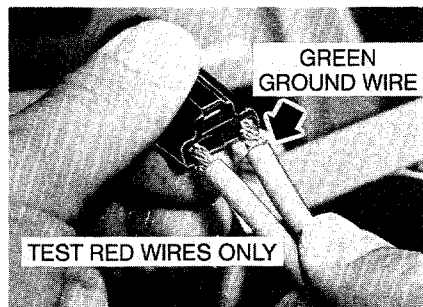
6-69: Use jumper wire to "jump" key switch wires.
